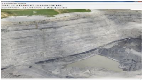
Left: Overlay of UAV ortho and 3D point cloud data from a mining site in ArcMap.
